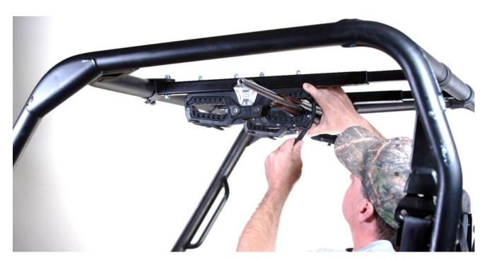
7. Re-Fasten the rubber retention straps, choose whichever hole provides the desired compression and make sure gun is secure before operating the vehicle.
