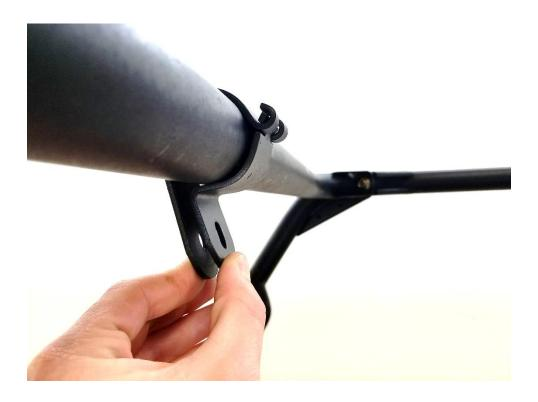
2. Place a metal P clamp around the forward upper roll cage tube.
