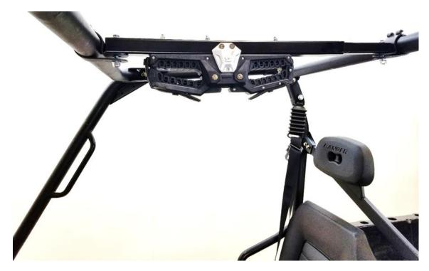
4. Place another metal p clamp around the rear overhead roll cage bar and fasten the slider tube to the p clamp using the supplied M10x50 bolt and nut. Keep loose at this time
