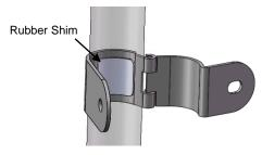
Use 1 shim on the inner half to adapt the 1.75" roll cage clamp down to 1.625" and do the same to adapt the 2" clamp down to 1.875"
