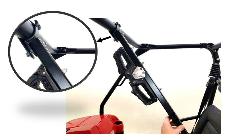
3. Take the gun grip assembly with slider tube inserted (tighten rattle prevention bolt so the slider tube doesn't fall out) and mount to the p clamp using the supplied M10x50 bolt and nut. Keep loose at this time.
