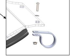
6. Insert bolt through washer and windshield, loosely install nuts on both top clamps.
