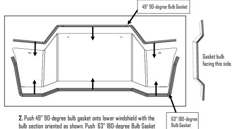
bulb section oriented as shown. Push 63" 180-degree Bulb Gasket onto lower windshield.
