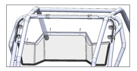
**9.** Insert lower windshield. It should fit snuggly against rear speakers, behind seat belt, and against upper windshield.
