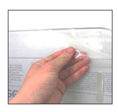
1. Peel plastic 4"back on edges of windshield. Remove completely after windshield is fully installed.
