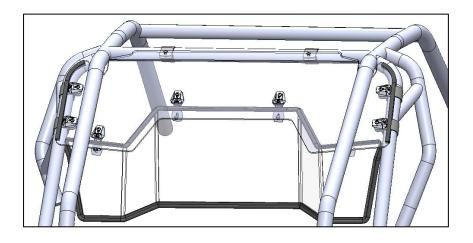
12. The bracket slots allow for adjustment in the lower windshield so that you may ensure the windshield gasket seals along bottom edge. Make sure windshield is centered and snug, tighten all bolts.
