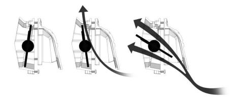
The vent has 3 positions: Closed, Defog, and open.
