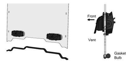
2. Push the gasket on the bottom of the windshield with the bulb section oriented as shown
