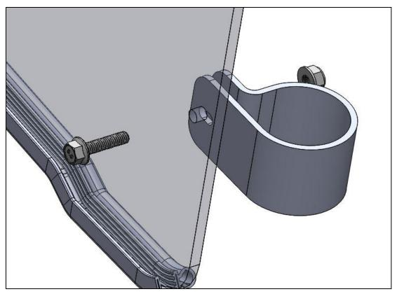
2. Snap 9 P Clamps onto the roll cage, 3 on each side with the flanges facing forward, and 3 across the top in the approximate locations of the mounting holes in the windshield. Mount windshield with the 9 bolts and nuts. Move windshield around as necessary for alignment before fully tightening.
