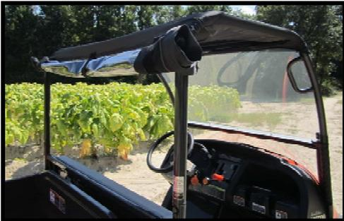
**A** – The rear window can be rolled up by undoing step 2, rolling the window up from the bottom, and securing with the three straps at the top of the window as shown.
