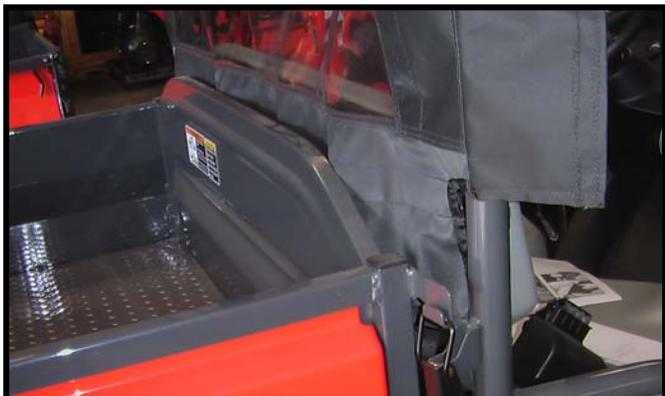
4. Allow the back side to drape between the dump bed and the seat.
