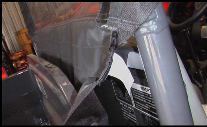
5. Locate the velcro at the base of the soft top with the adhesive velcro strip. Remove the backing to the adhesive and adhere to the horizontal rectangular bar behind the seat..
