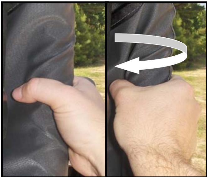
2. Locate the velcro straps running down the length of the rear vertical ROPS bar. Fasten around the bar. Repeat this step for the opposite side.
