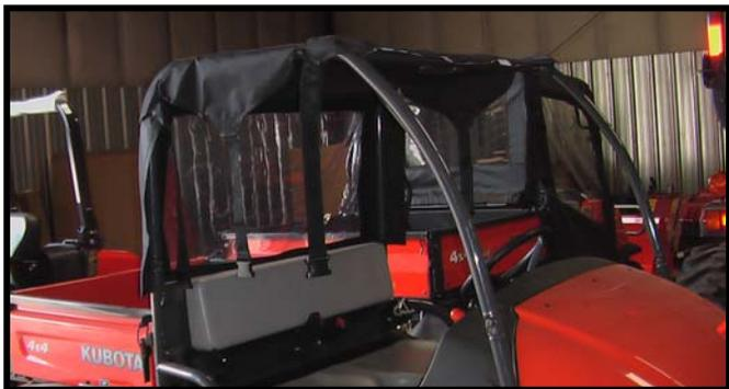
1. Lay the soft top over the roll cage of the vehicle making sure the straps are on the outside of the ROPS.
