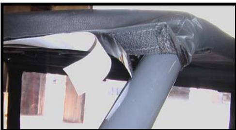
**B** – The velcro strip along the front of the soft top is so it can be attached to a windshield by removing the adhesive backing and adhering the velcro to the top of the windshield.
