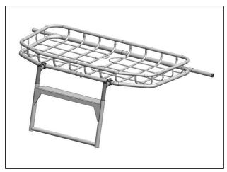
2. Attach the riser assembly to the front of the hood rack and bolt the (2) front riser caps in place. Snug the cap bolts, but keep them loose enough to allow rotation.
