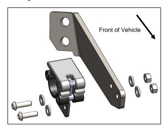
**3**. Attach the two clamps (E) to the roll cage clamps (G) with two M6 x 16mm socket head bolts, 4 washers and 2 nuts. The clamp lever should open towards the front of the vehicle.
