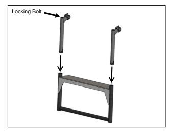
1. Note the riser orientation shown above. Insert the (2) Riser stems (C) into the front riser/light mounting Plate (D) a few inches in. Tighten the locking bolt at the top of the tube with allen wrench just enough to hold the riser stems in place. You will tighten after final assembly.
