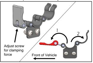
To open a clamp, lift up on both levers in the order above. Orient all clamps so the first clamp lever opens towards the front of the vehicle. To increase clamping force, tighten screw; to decrease the clamping force, loosen screw before locking.
