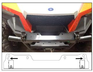
2. Line up the holes on the bumper mount and place on top of the bumper. Bolt together with M8x30mm hex head bolts, washers, and M8 locknuts. Make sure the spacers are between the bumper mount and bumper.
