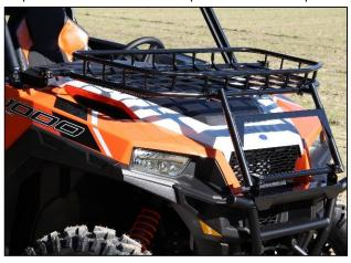
**4.** Open all four clamps and place basket assembly on the on the clamps. Lock all four clamps.
