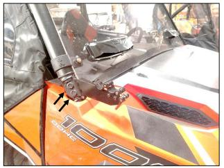
**3.** Undo the two roll cage bolts holding the A pillers of the vehicle together, and use these bolts to bolt the roll cage mounts to the vehicle. The clamps should open towards the cab of the vehicle.
