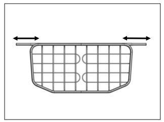
**5**. Adjust the width of the extendable tubes (G) so they stick out just past the clamps. (If necessary)
