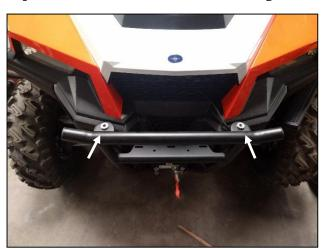
**1.** Place 2 metal spacers on the tabs on the bumper as shown above.
