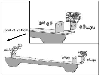
**4**. Attach the two clamps (E) to the bumper mount (F) using (4) M6 x 16mm bolts, (2) washers and (4) locknuts. Make sure all clamp levers open towards the front of the vehicle.
