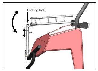
**6.** Adjust the hood rack angle by loosening the bolt on the front riser stems and pushing up or down on the front of the rack. Adjust clamps and brackets as necessary, then tighten all bolts. We recommend no more than 5% of slope to the hood rack.
