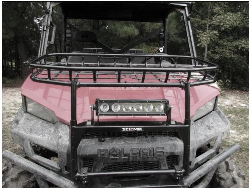
Lights or a light bar can be attached to the hood rack by drilling holes in the light mounting plate. We recommend our 13" 60 Watt Seizmik Light Bar with 5,400 Lumen output. Part Number #12037
