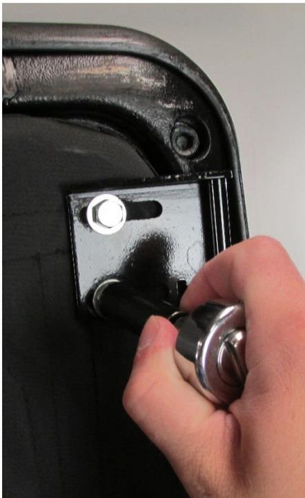
**24.** Move the door back into the closed position, again pressed firmly against the gasket on the bodywork. This may require you to move the striker assembly up or down in order for the latch to fully engage. At this point tighten the door plate bolts just enough to keep the door from sliding forward and back.
