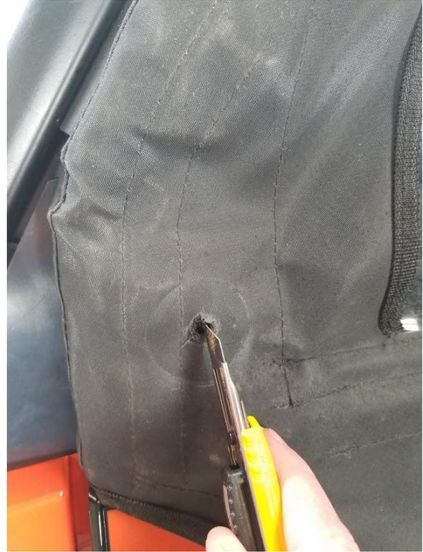
33. Using a sharp razor or utility knife, cut the textile so the mirror mounting bolt can pass through.
