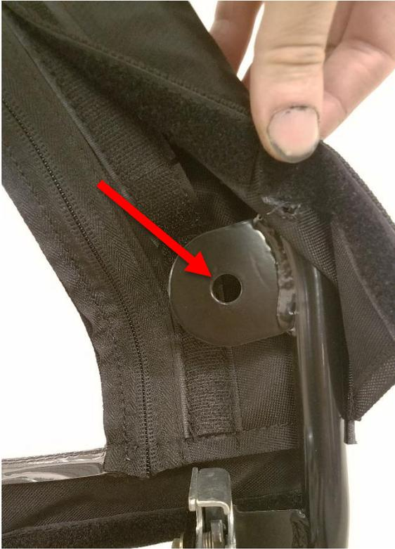
32. Locate the mirror mounting bracket on the inside of the door frame. Mark the location of the hole with a punch so that it can be seen on the outside of the door textile.
