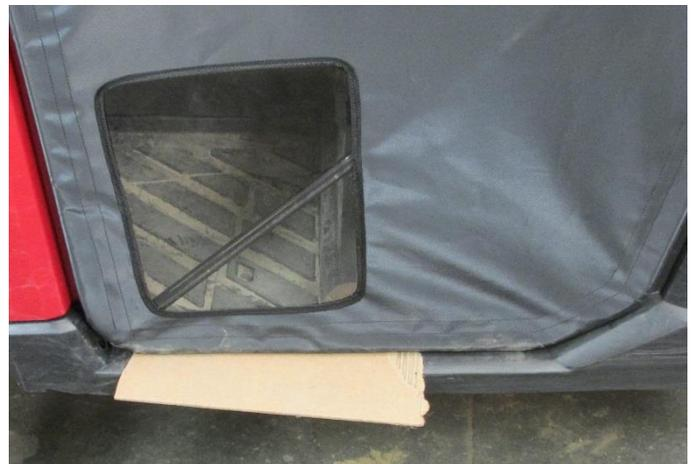
**21.** We have found that placing a piece of scrap cardboard at the bottom edge as shown will help line up the door so that it will not drag on the bodywork when the door is finished being adjusted.
