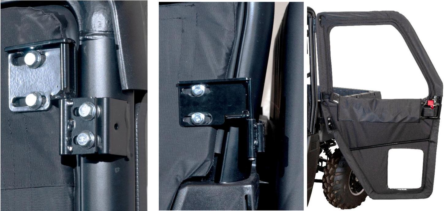
**19.** Insert the Sliding Hinge Pins into the Hinge Mount Barrels and roll down the window for easier adjustment. Rolling down the window will allow you to access and adjust the striker bolt and plate from the outside of the vehicle.
