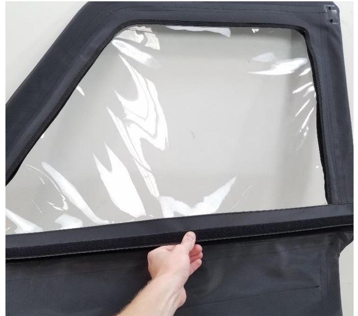
**14.** Pull Upper door textile down firmly and attach to loop Velcro located on the outside of the lower panel as shown.
