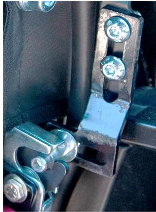
**5.** Attach striker bolt in the remaining slot on the Striker Plate in the orientation shown. Install with supplied nut. (This will adjust how far in and out the door is from the front of the body) (Do not fully tighten at this point.)
