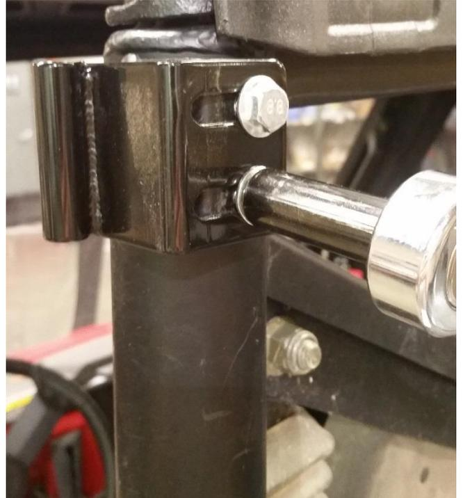
**30.** The Upper Hinge mount plate may be adjusted in and out to affect how much the door will compress the gasket.
