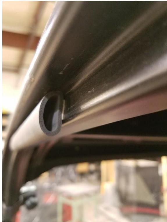
**18.** Clean the highlighted area of the ROPS structure and bodywork with rubbing alcohol or window cleaner. **(Failure to clean ROPS structure and bodywork will result in gasket falling off and doors not sealing properly!)** Adhere the provided gasket into the outer channel of the roll cage as shown by the highlighted area above. Be sure the gasket is oriented the same as the image above.
