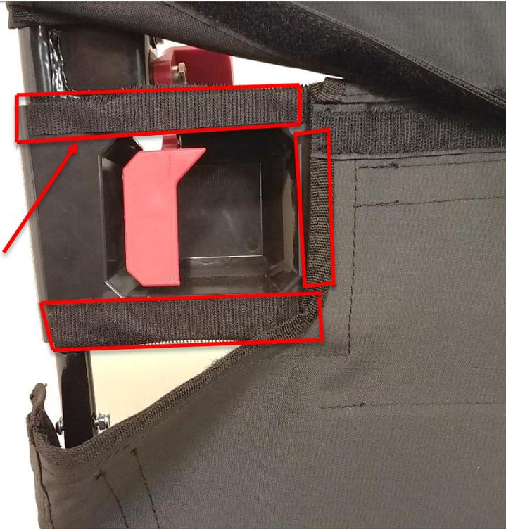
**13.** Clean plastic with alcohol or degreaser, then place pieces of 1" wide adhesive hook Velcro onto plastic molded pocket in the areas outlined. This will keep the upper door textile secure at the front of the door.
