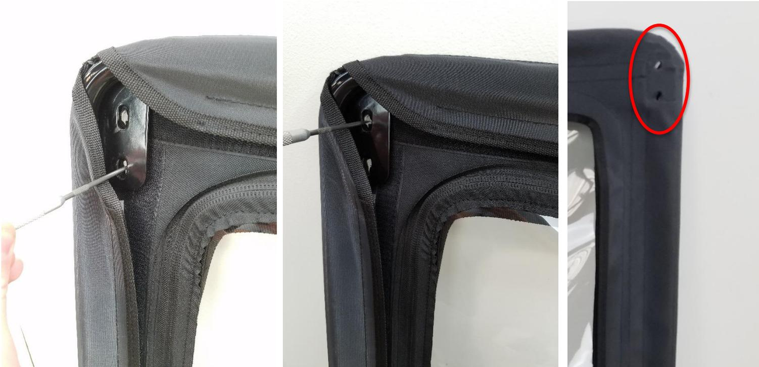
**16.** Holes need to be cut in door textile panels in order to mount the Upper and Lower Sliding Hinges. **Ensure textiles are tight and fit as desired before marking and cutting holes.** Take a sharp scribing tool and punch a small hole through the textile indicating the center of the slot. Take a razor blade and carefully cut out the small amount of textile so that the supplied M8 bolt may pass through the plate and the textile. Repeat this process for the lower mounting location.
