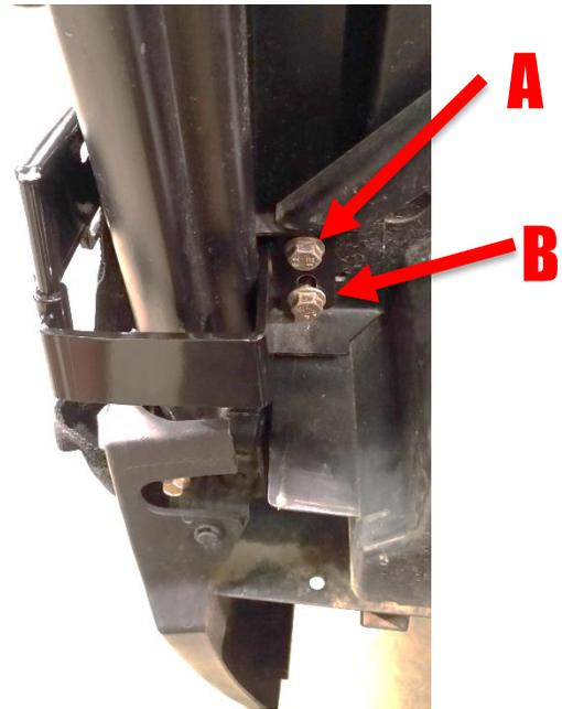
**3.** Locate the factory bolts at positions "A" and "B". These will be used to attach the Lower Hinge Plate. Remove fasteners. (Seat back plastics may need to be removed or loosened to gain easier access to the nuts.) Place bracket as shown and reinstall bolts and nuts.
