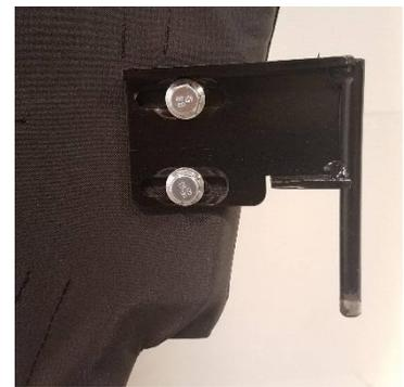
**17.** Pass M8x25mm bolts through the Upper Sliding Hinge, textile, then the welded on door plate. Attach using M8 washers and lock nuts as shown. Repeat steps for Lower Sliding Hinge using M8x25mm bolts, M8 washers and lock nuts. Do not fully tighten at this time. Sliding Hinges are slotted for door adjustment.
