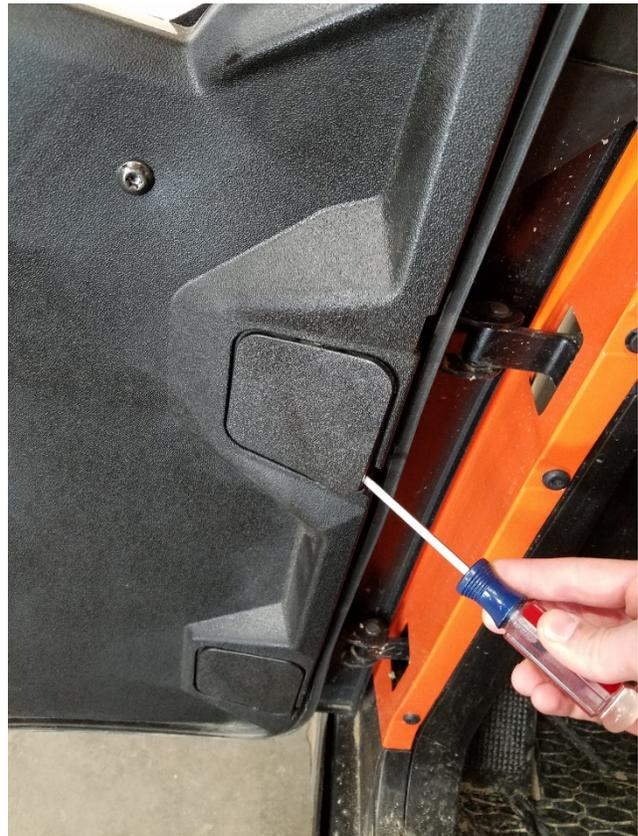
2. Use a flat blade screwdriver to remove the hinge adjustment covers to reveal the last two Torx fasteners (top and bottom). Remove the inner door Panel
