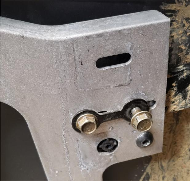
3. Remove the upper door hinge mounting bolt closest to the vehicle as shown above (you will re-use this bolt later).
