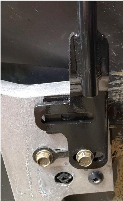
5. Insert the front spacer block between the Front Mounting Bracket (B) and the aluminum Polaris door frame.
