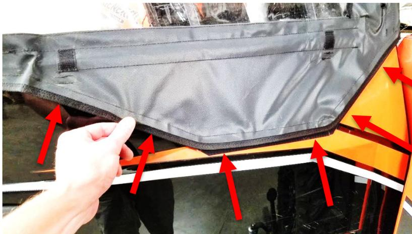
**21.** Lay the Textile Flap over the outer door plastics and mark the location of the outside perimeter. Clean the designated area with rubbing alcohol or window cleaner.
