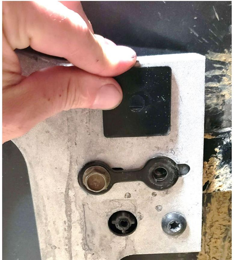
4. The front spacer (D) ensures the Front mounting bracket (B) is installed with the correct offset so that the pins on the upper door frame line up with the bracket.
