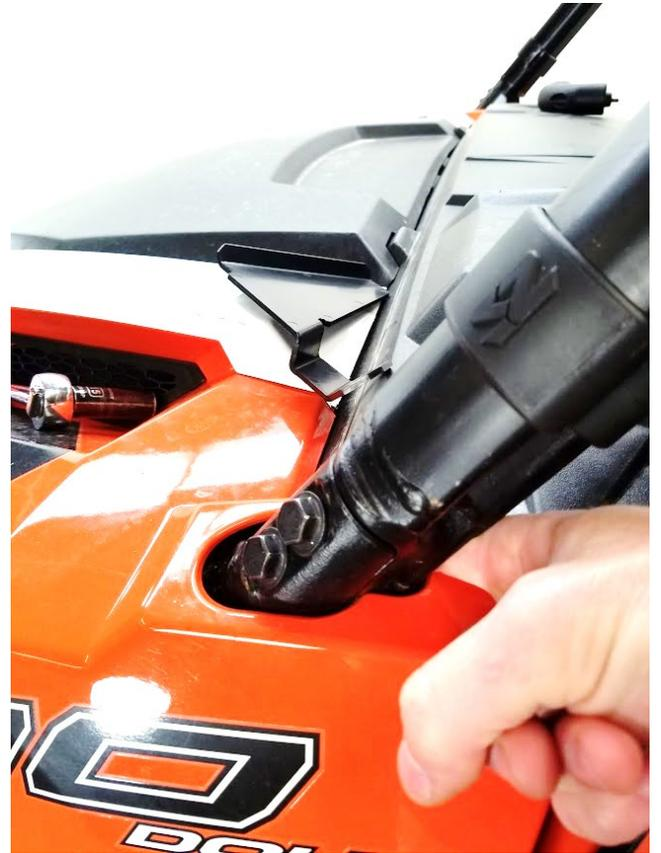
**TIP:** Be sure to keep a finger or have a friend hold the nuts in place or they will fall and possibly be hard to locate. A magnet can be your friend here.
