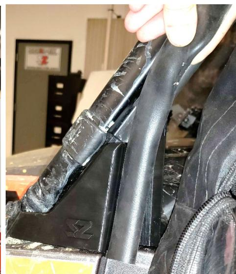
**20.** Clean the highlighted area of the roll cage and filler panel with rubbing alcohol or window cleaner. Adhere the provided gasket into the outer channel of the roll cage as shown by the highlighted area above. Be sure the gasket is oriented the same as the image above.
