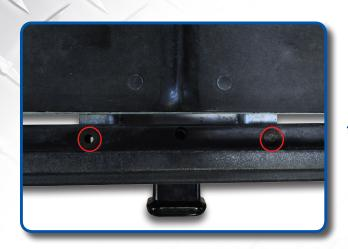
Using hardware retained from Step 1, attach bumper. Retained hardware should mount down from bumper through trailer hitch. Tighten hardware.
