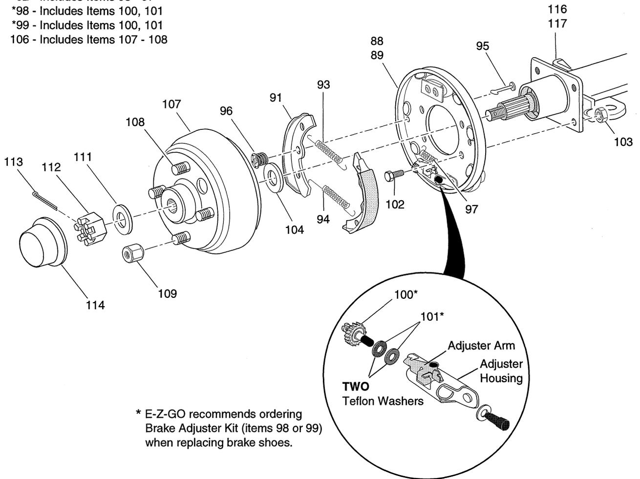
\* E-Z-GO recommends ordering Brake Adjuster Kit (items 98 or 99) when replacing brake shoes.
