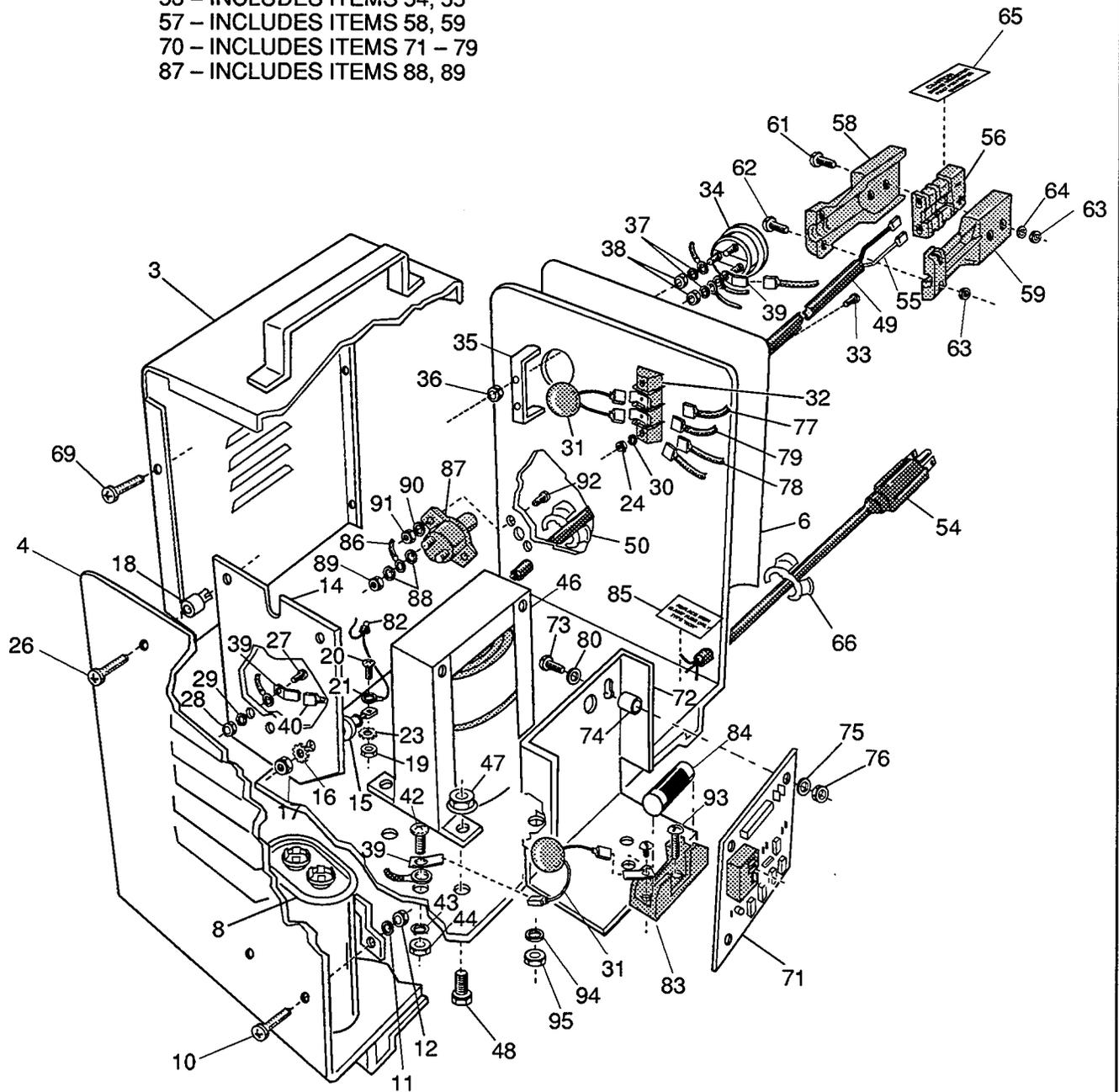
**BATTERY CHARGER, TOTAL CHARGE<sup>®</sup> III (PORTABLE) ELECTRIC POWERED TRUCK**
