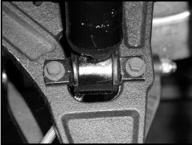
Figure 7-35 Front Shock Bottom Mount
