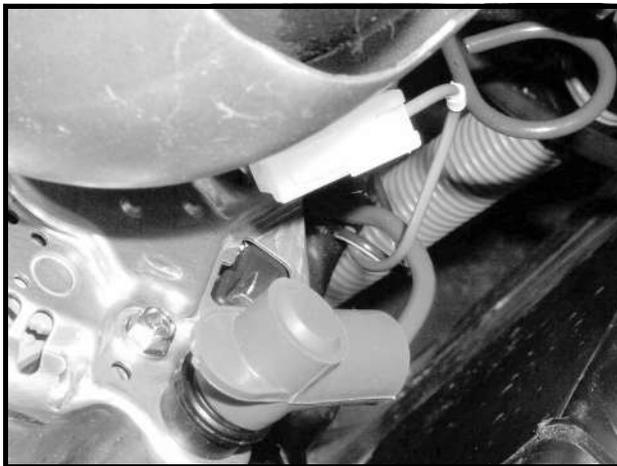
Figure 12b-11 18-Gauge Purple Wire at Alternator
