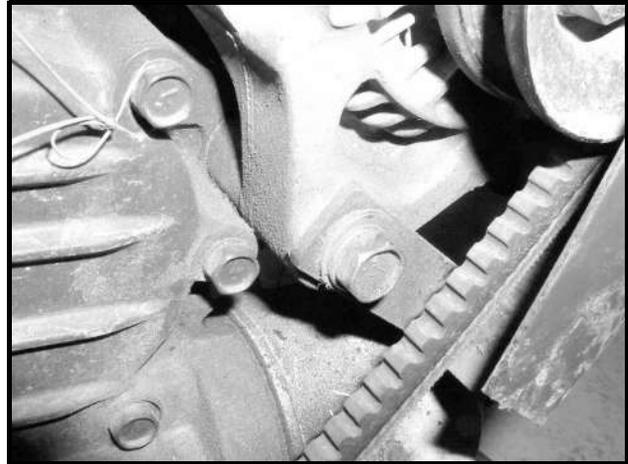
Figure 12b-14 Alternator Mounting Bolt
