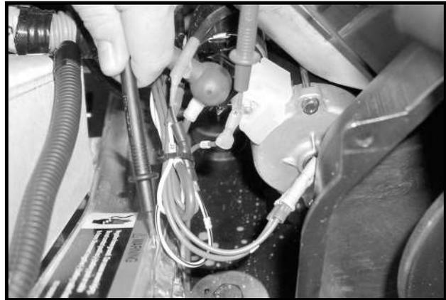
Figure 11a-11 Starter Circuit Test
