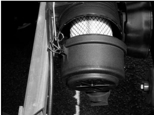
**Figure 13b-29 Air Filter Cartridge**
