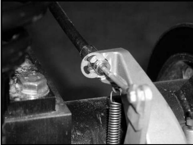
Figure 6-22 Park Brake Cable Attachment
