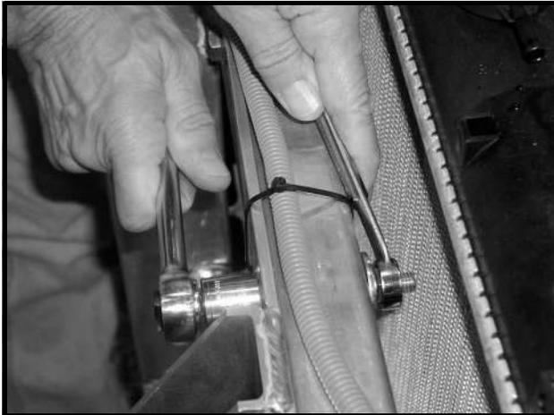
**Figure 15-11 Top Front Frame Bolts**
