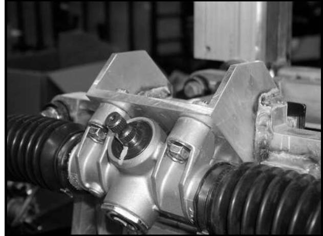
**Figure 7-6 Rack and Pinion Bolts**
