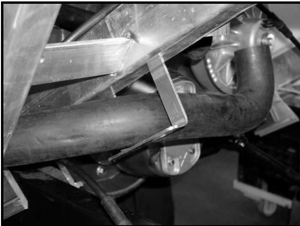
**Figure 13b-31 Air Intake Support Bracket**
