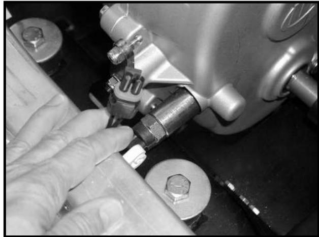
Figure 14-19 Neutral Sensing Connector
