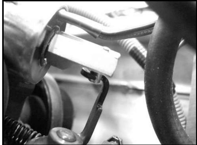
Figure 12b-4 Fuel Solenoid Lever
