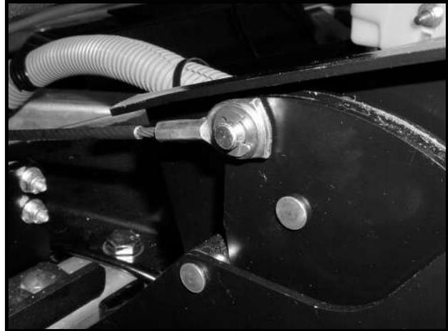
Figure 6-26 Park Brake Pedal Assembly
