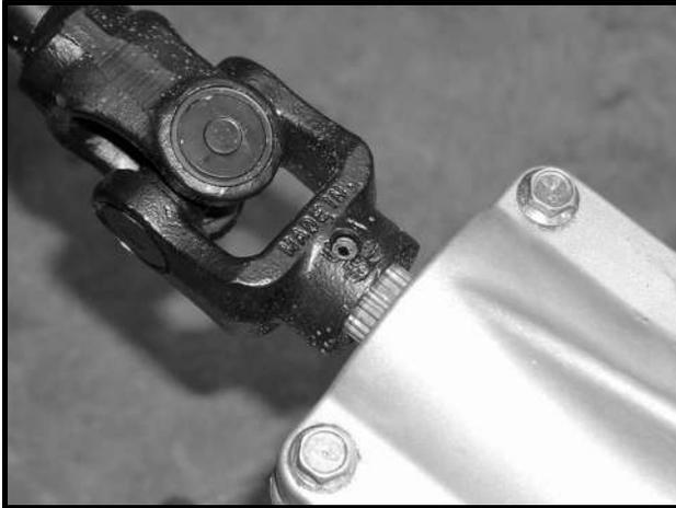
Figure 14-8 Roll Pin in Front Drive Shaft
