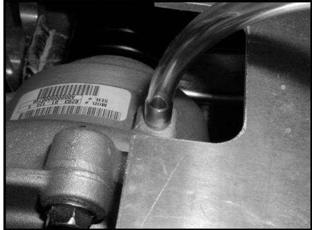
Figure 14-9 Differential Vent Tube
