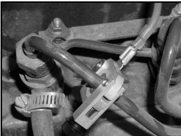
Figure 13b-25 Diesel Probe Fuel Line Clamp On Engine
