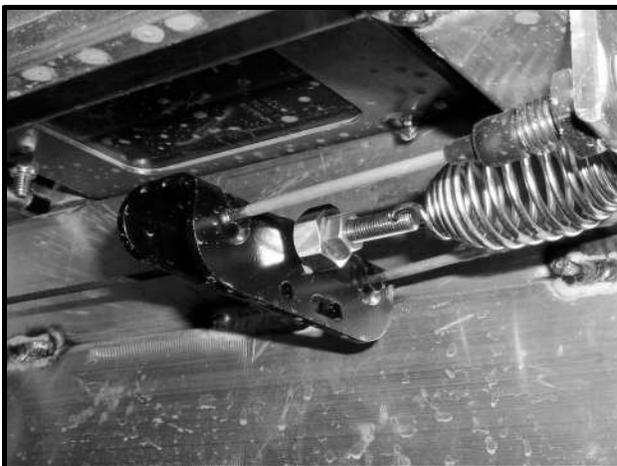
**Figure 5-6** Park Brake Adjustment Nuts
