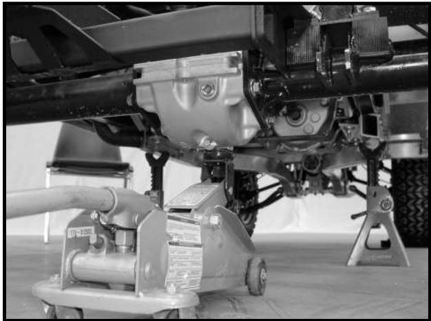
Figure 14-16 Position Floor Jack Under Differential
