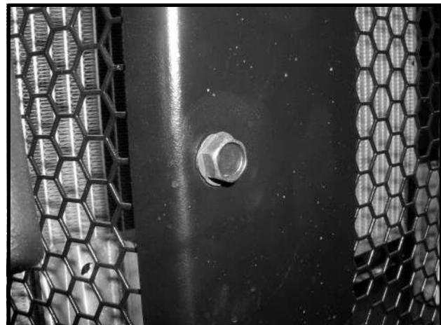
**Figure 15-6 Radiator Guard Front Bolts**
