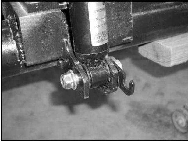
Figure 14-17 Lower Driver Side Shock Mount
