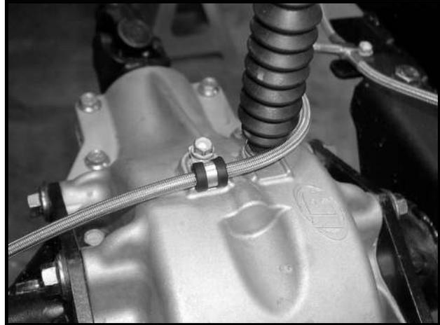
**Figure 14-14** Rear Differential Brake Line P-Clamp
