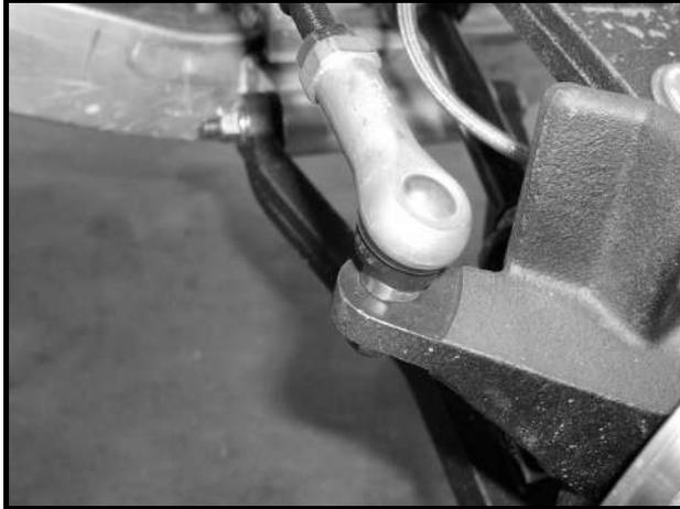
**Figure 7-5 Drag Link Ball Joint**
