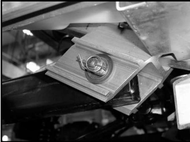
Figure 9-3 Swing Arm Bolt, Nut and Rue Pin
