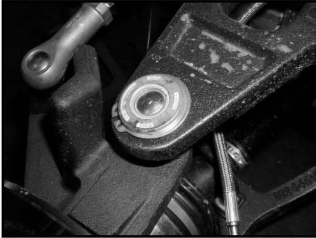
Figure 7-31 Ball Joint C-Clip
