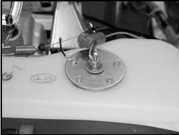
Figure 13a-9 Fuel Level Sensor
