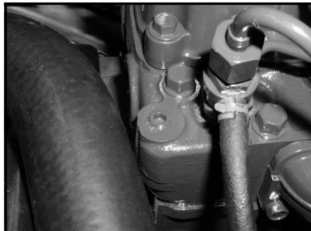
**Figure 15-2 Engine Block Coolant Plug**
