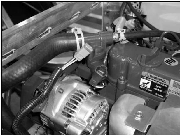
Figure 12b-16 Thermostat Switch
