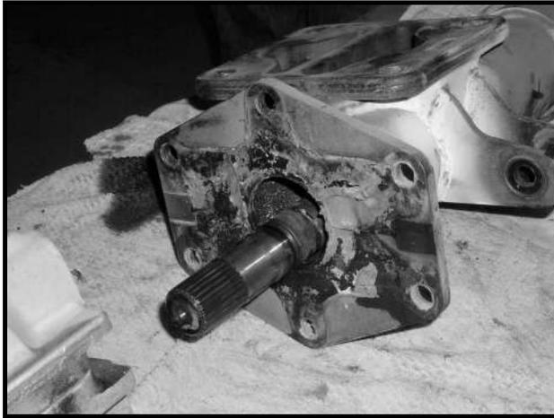
Figure 14-25 Separate Axle Tube from Differential
