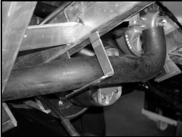
Figure 13a-28 Air Intake Support Bracket
