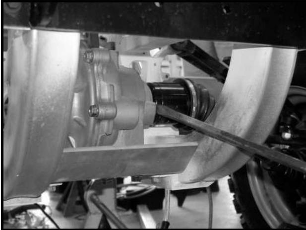
Figure 14-5 Separate Half Shaft from Differential
