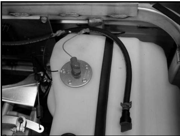
Figure 13a-8 Gasoline Fuel Tank
