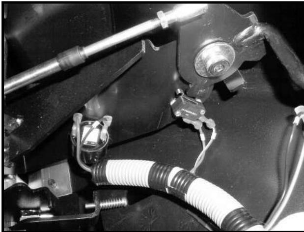
**Figure 11a-25 Reverse Warning Buzzer and Limit Switch**
