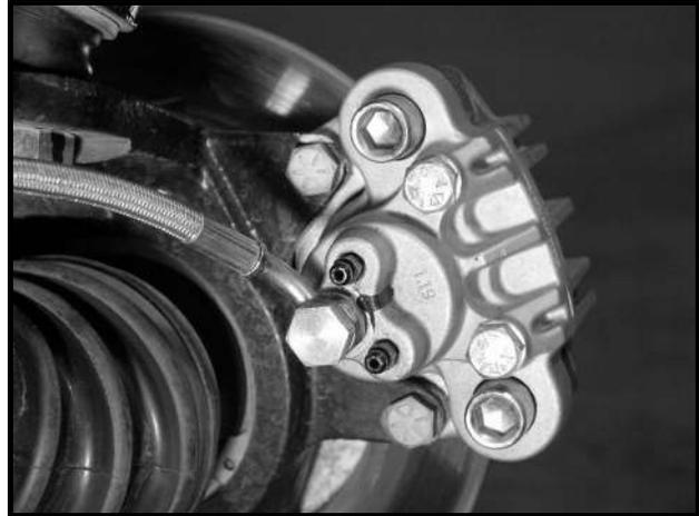
Figure 6-4 Front Brake Line and Banjo Bolt
