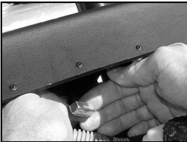
**Figure 12a-12 Bed Lift Circuit Breaker**
