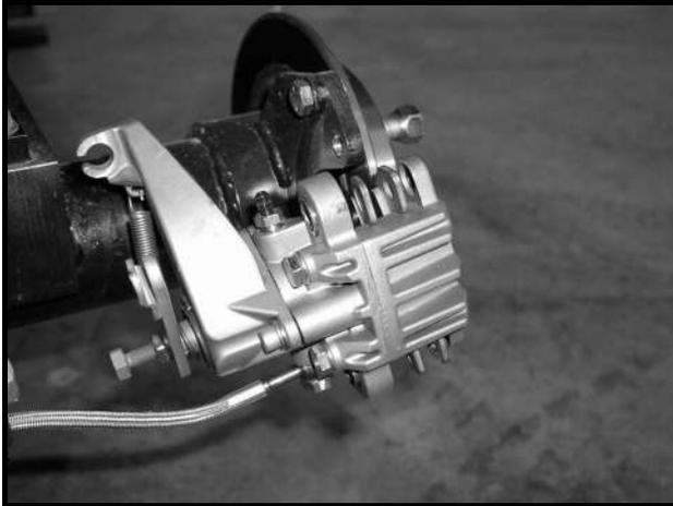
Figure 6-5 Rear Brake Pad and Caliper
