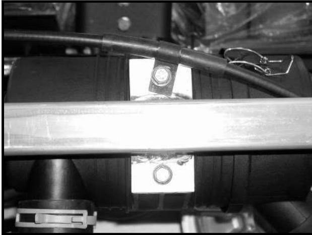
**Figure 6-24** Air Filter and Park Brake Cable Clamp
