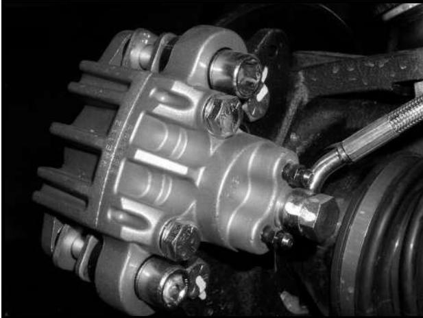
Figure 6-3 Front Brake Pad and Caliper
