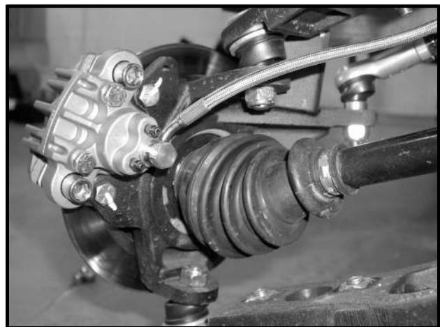
Figure 6-8 Brake Caliper and Upright
