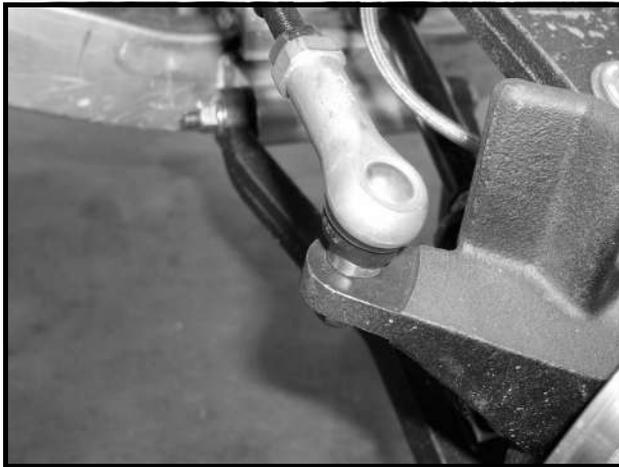
**Figure 7-26 Drag Link Ball Joint**
