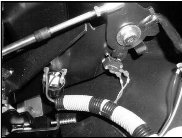
Figure 12a-6 Reverse Warning Buzzer and Limit Switch
