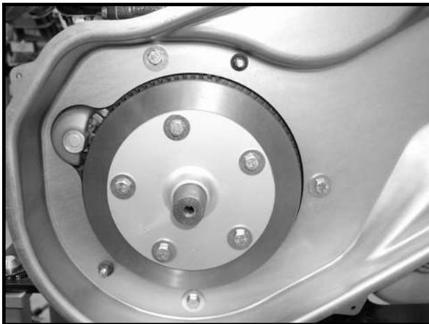
Figure 13b-40 Inner Cover Hardware on Diesel Engine
