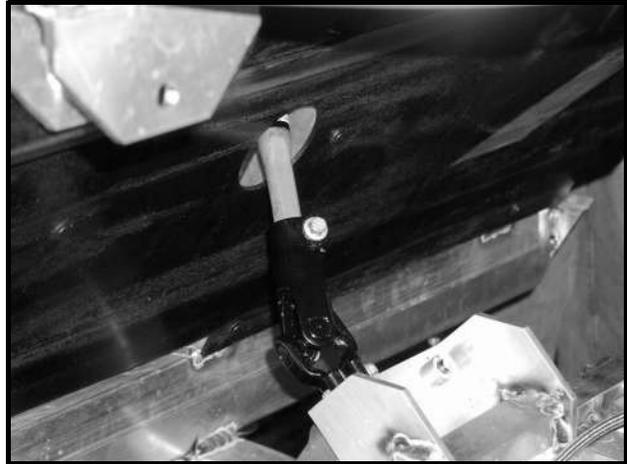
Figure 7-4 Steering Universal Joint
