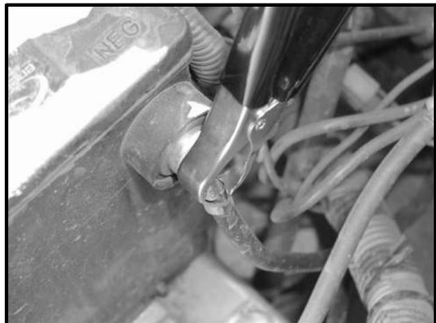
Figure 13b-26 Diesel Probe Battery Cable Clamp
