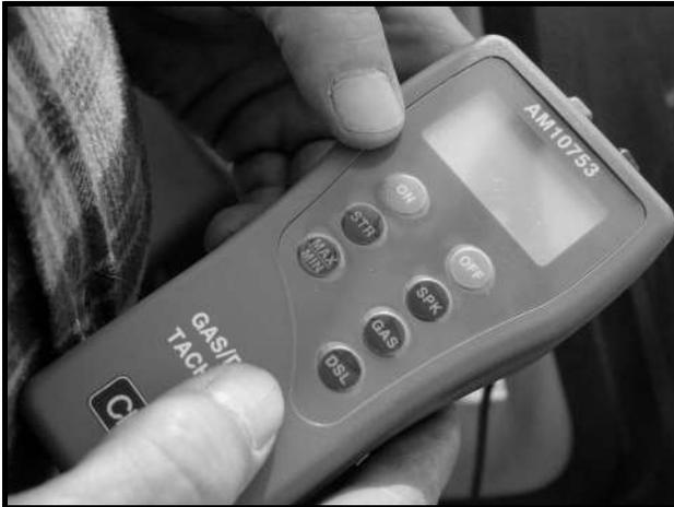
Figure 13b-23 Tachometer For Engine RPM
