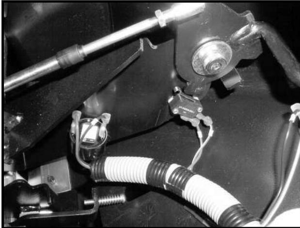
Figure 11b-33 Reverse Warning Buzzer and Limit Switch
