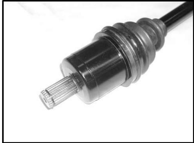
Figure 14-6 Compression Ring on Spline
