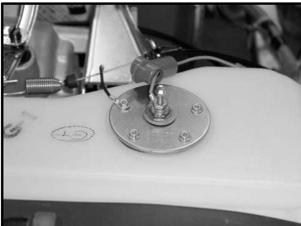
**Figure 13b-19 Fuel Level Sensor**
