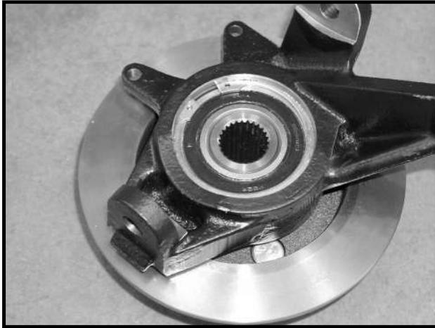
Figure 6-16 Upright, Bearing and Shaft Assembly
