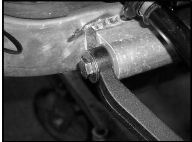
Figure 7-33 A-Arm Frame Bushings
