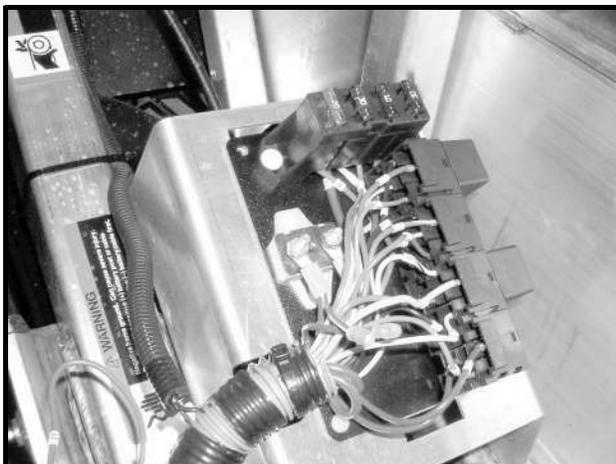
Figure 11b-24 Differential Relay Removed
