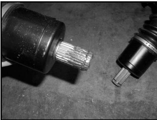
Figure 14-7 Apply Anti-Seize to Splined Ends
