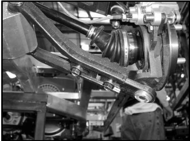
Figure 14-4 Camber Adjustment Bar
