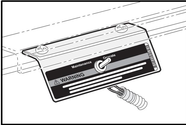
Figure 13 Neutral Lockout Switch
