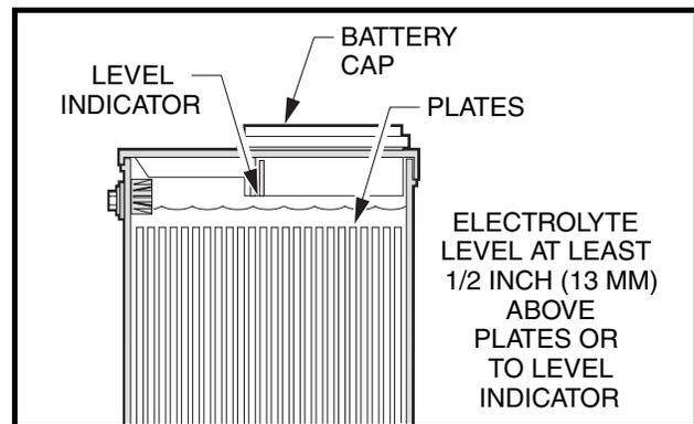
Figure 28 Gasoline Battery Electrolyte Level
