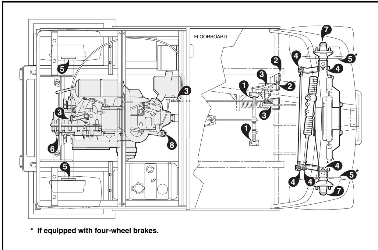
Figure 22 Lubrication Points – Gasoline Vehicles
