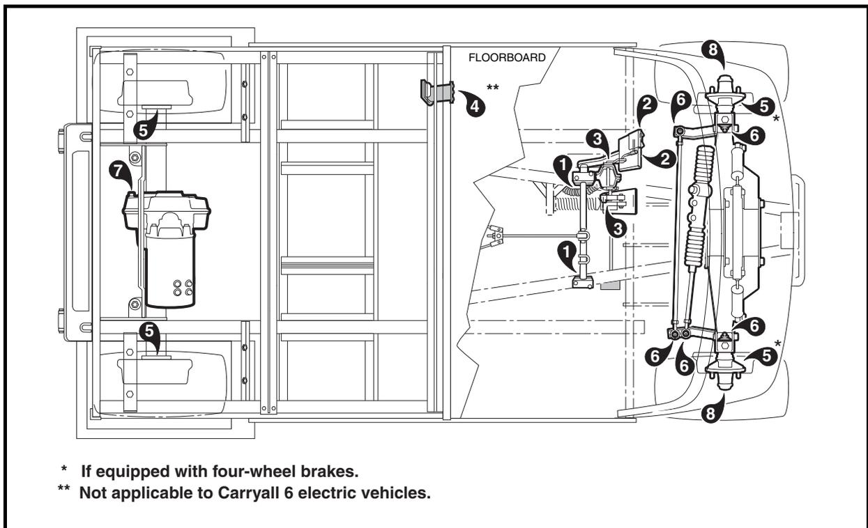
Figure 21 Lubrication Points – Electric Vehicles
