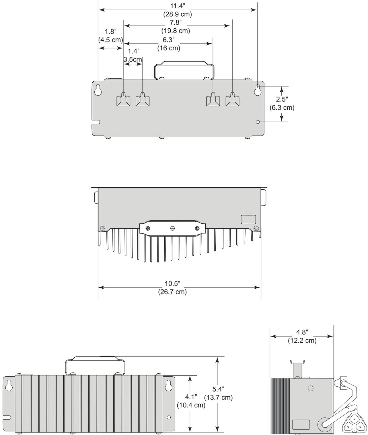
**Fig. 3 Battery Charger Dimensions**
