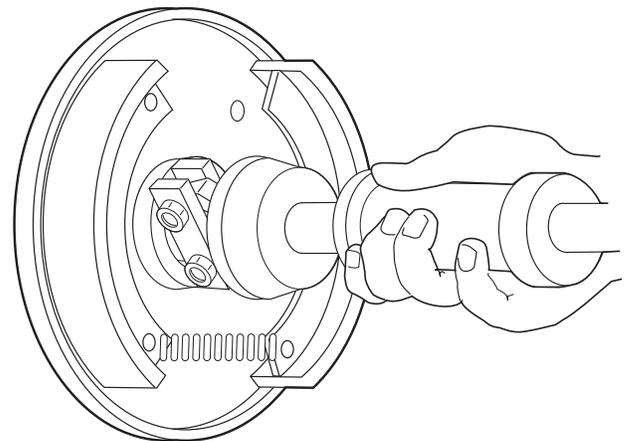
**Fig. 6 Removing Seal**
