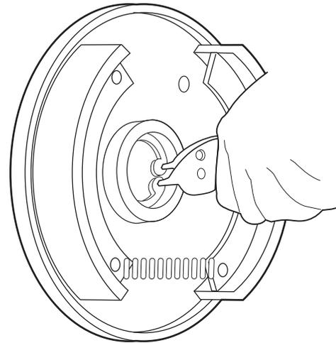
**Fig. 5 Removing/Installing Inner Snap Ring**
