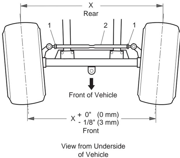
**Fig. 4 Wheel Alignment**
