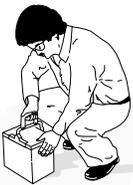
Batteries are heavy. Use proper lifting techniques when moving them. Always lift the battery with a commercially available battery lifting device. Use care not to tip batteries when removing or installing them; spilled electrolyte can cause
