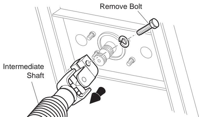
**Fig. 5 Disconnect Intermediate Shaft to Center Steering Wheel**
