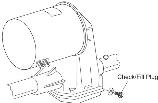
Fig. 1 Add, Check and Drain Rear Axle Lubricant
