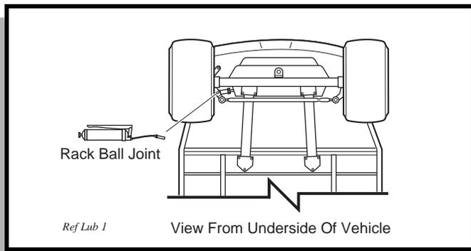
Fig. 2 Lubrication Point
