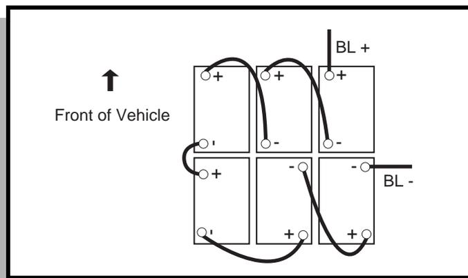
Fig. 1 Battery Connections
