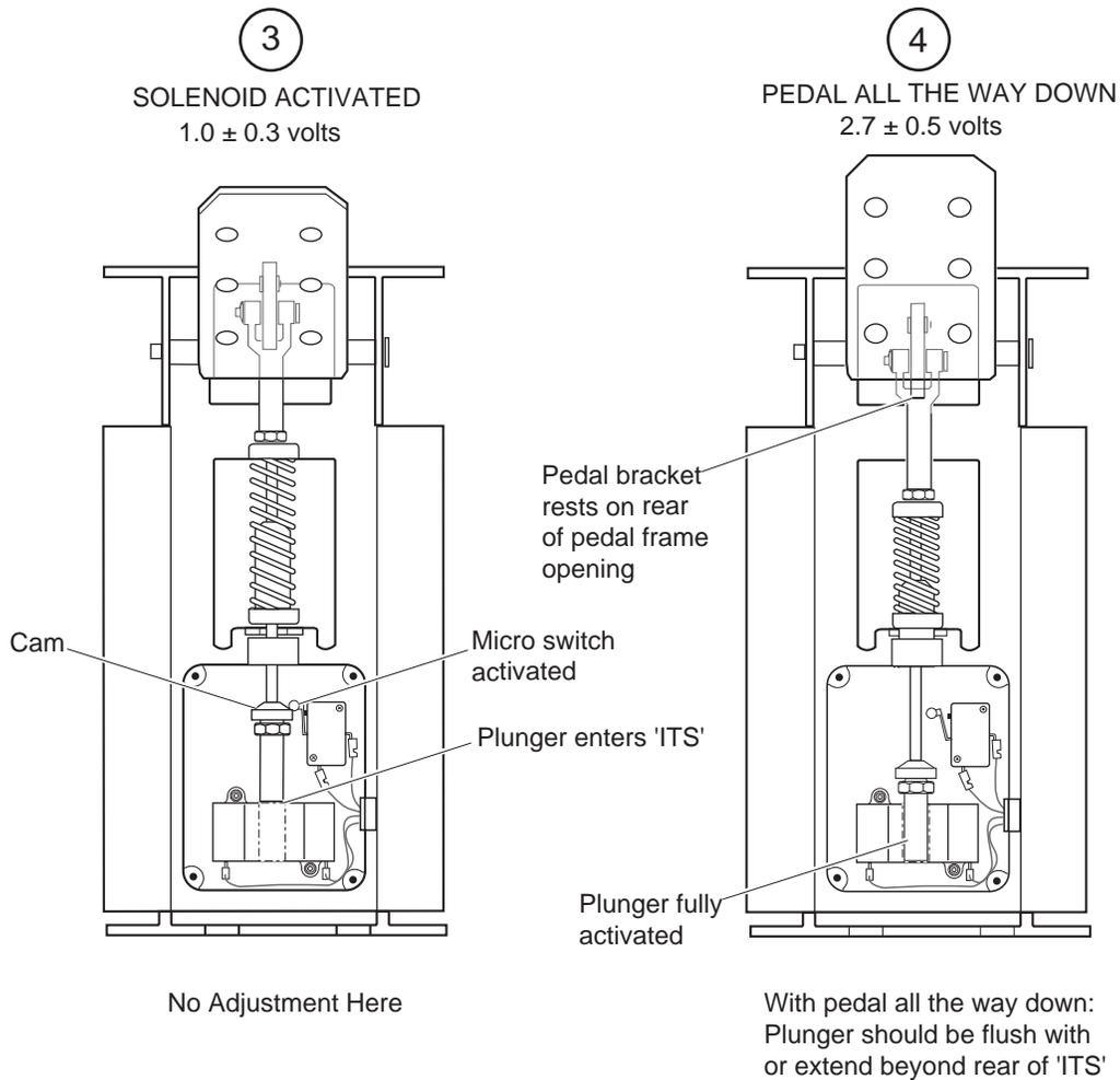
**Fig. 12 ITS Adjustment (Sheet 2 of 2)**
