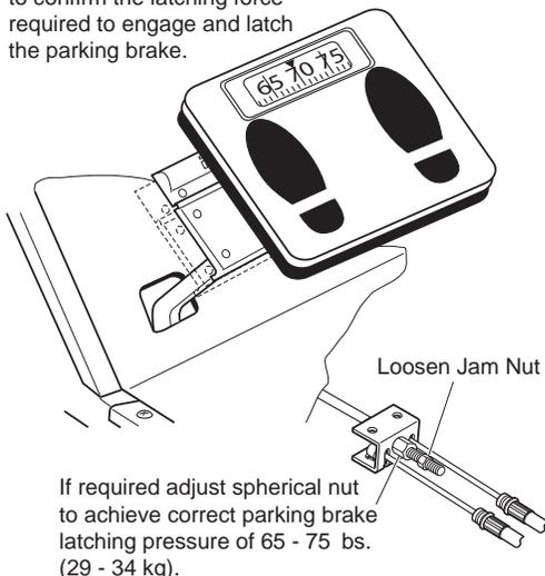
**Fig. 20 Checking Parking Brake Latching Pressure**
