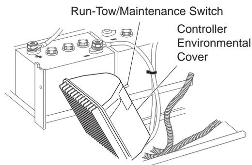
Fig. 1 Run-Tow/Maintenance Switch
