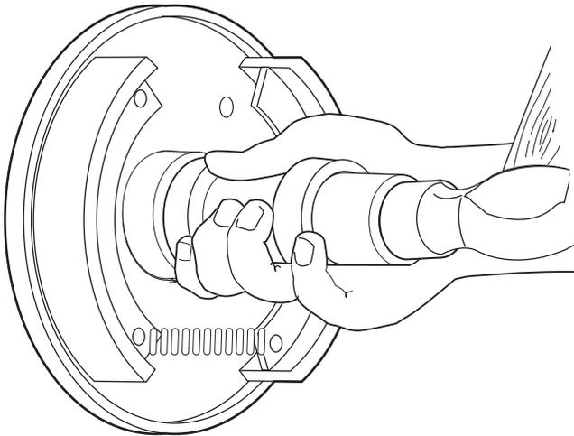
**Fig. 7** Installing Seal
