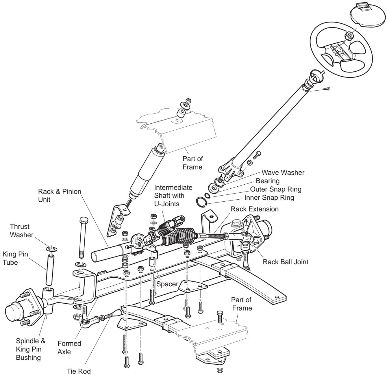
**Fig. 1 Axle Mounted Steering and Front Suspension**
