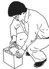
Batteries are heavy. Use proper lifting techniques when moving them. Always lift the battery with a commercially available battery lifting device. Use care not to tip batteries when removing or installing them; spilled electrolyte can cause burns and damage.
