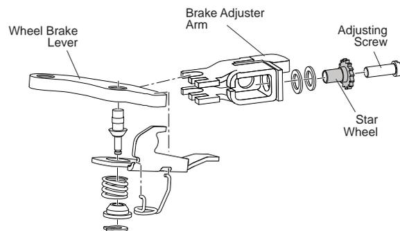
Fig. 15 Adjuster Mechanism
