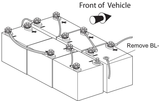
**Fig. 1 Disconnect Battery Cable**
