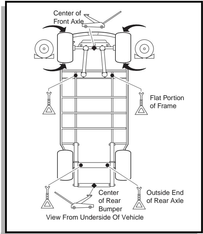
**Fig. 2 Lifting the Vehicle**
