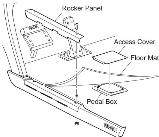
Fig. 2 Access to Pedal Box
