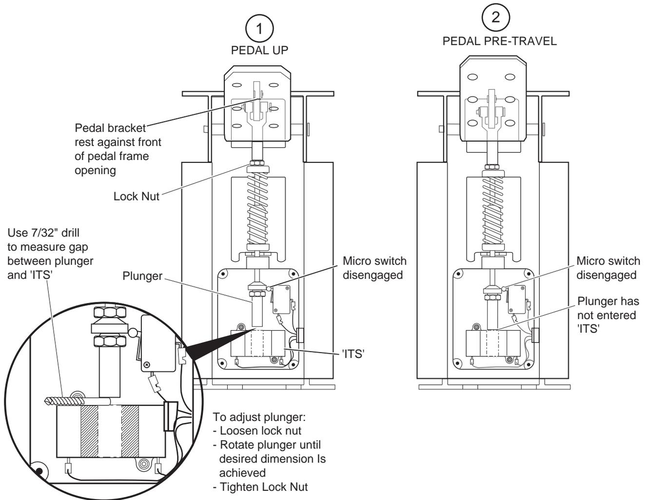
**Fig. 11 ITS Adjustment (Sheet 1 of 2)**
