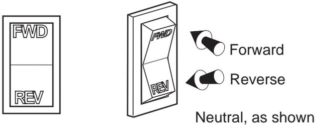
Fig. 1 Direction Selector Switch
