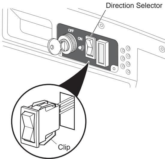
**Fig. 2** Direction Selection Switch Replacement
