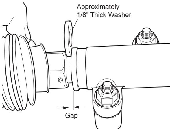
**Fig. 19 Checking Gap**
