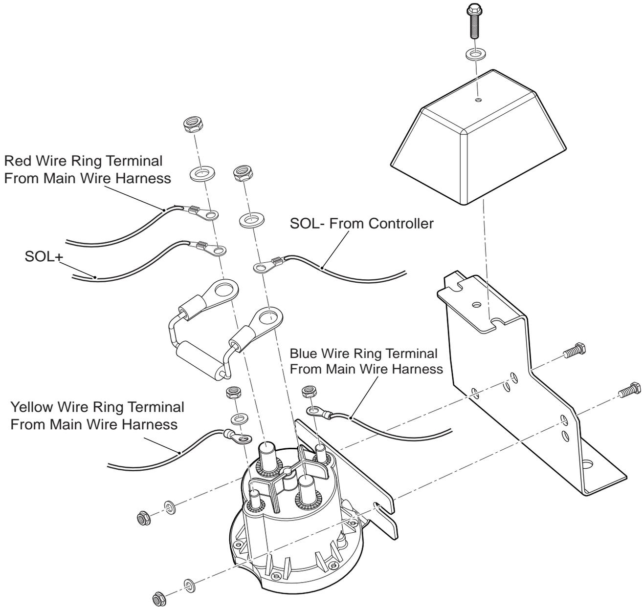
**Fig. 13 Solenoid Wiring**
