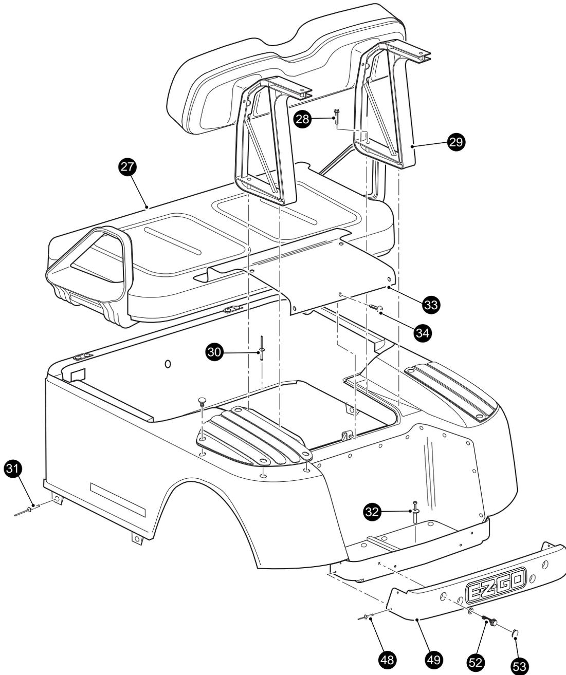
**Fig. 3 Body Components (Rear)**
