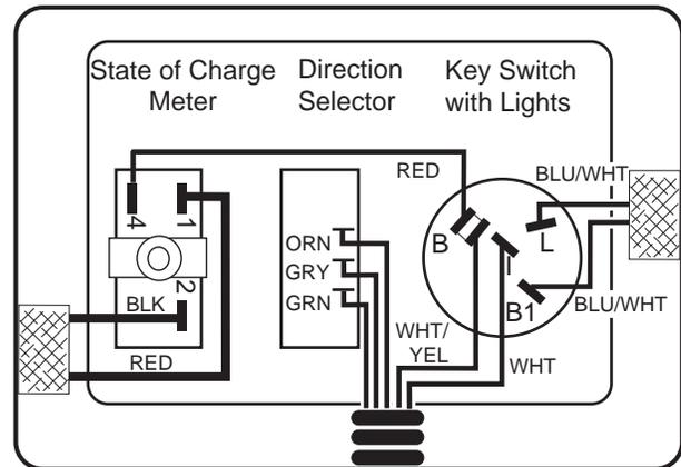
**Fig. 3** Direction Selector Switch Connections
