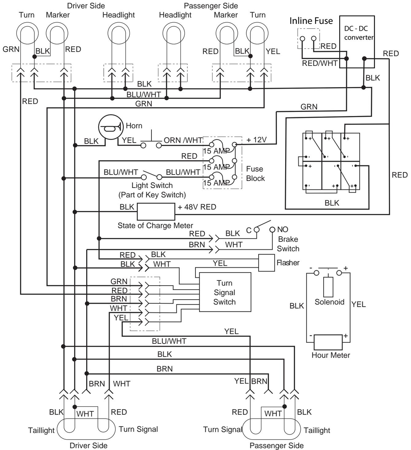
For vehicles without turn signals, remove WHT wire from left rear turn signal
