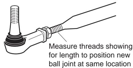
Measure threads showing for length to position new ball joint at same location
