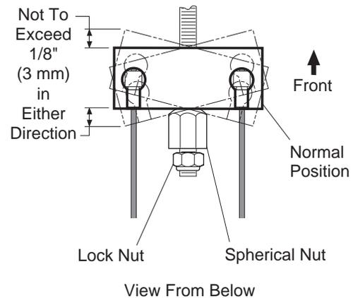
NOTE: This dimension is factory pre-set with the parking brake disengaged and is not to be changed.
