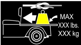
SECURE LOAD AS FAR FORWARD AS POSSIBLE. MAXIMUM LOAD BED CAPACITY
