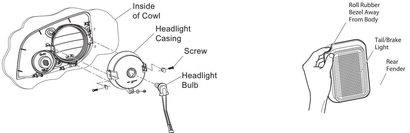
To replace the tail and brake light bulb, roll the rubber bezel from around the edge of the taillight and remove lens. Install replacement bulb and replace lens.
