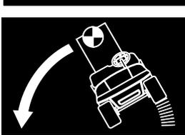
LOAD WITH HIGH CENTER OF GRAVITY COULD RESULT IN TIP OVER
