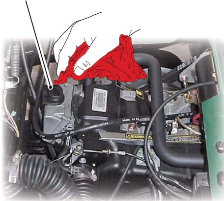
Clean the area around filter. Using a filter wrench, strap wrench or other suitable wrench, remove the filter (B) from the engine and allow the oil to drain. The 'O' rings may remain on engine (A) or filter (B)
