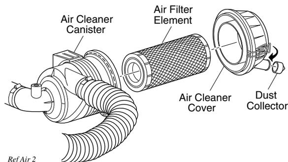
If the element is in acceptable condition, loose dirt may be removed by tapping the filter lightly. Do not use oil on the filter element or any part of the unit.
