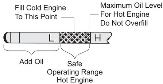
The engine can be operated safely as long as oil is within the safe operating range as indicated on the dip stick. **Do not operate vehicle if oil level is below the safe area indicated on the dipstick.**
